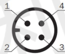
Connector plug, M12 x 1,4-pin,A-coded
